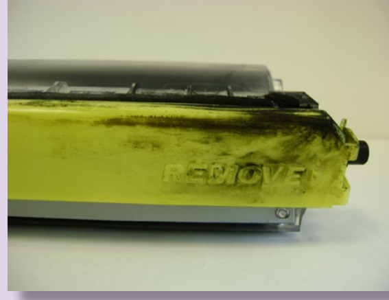
Example of toner leakage with a newly opened aftermarket cartridge.
