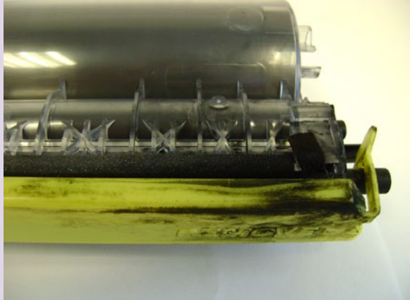
Example of toner leakage with a newly opened aftermarket cartridge.
